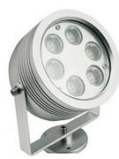
Power:6W Voltage:DC24V 50~60Hz Color: Red/ Green/ Blue/Yellow/White LED Type:6pcs \*High Power Size:D92XH180 Material: 6063 Aluminum IP Rate:IP65 Beam Angle:15° /25°/45° /60°
