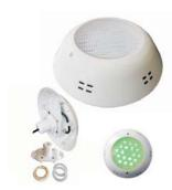
Power:25 W Voltage:AC/DC12V Color: White, Red, Green, Blue, Yellow. RGB LED Type:High Power Size: Ф290mm x H150.60mm Material: ABS + Transparent PC cover(lens) IP Rate:IP68 Beam Angle:15°/25°/30°/45°/60° Packing:10PCS/Carton
