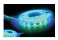
Power:7.2W Voltage:12V DC Color: FULL COLOR LED Type:5050SMD RGB Size:5000\*12\*2.4mm IC Type:INK1003 IP Rate:IP20/IP67 Packing:5 M/Roll, 3 leds/cut
