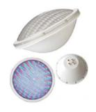
Power:18W Voltage:AC/DC12V Color: White, Red, Green, Blue, Yellow. RGB LED Type:315 PCS \* SMD3528 LED chip Size:⊕177mm x H105mm Material:Plastic + Transparent PC cover IP Rate:IP68 Beam Angle:120° Packing:20PCS/Carton
