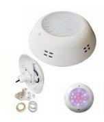
Power:19±1W(W/G/B)/18±1W(RGB)/14±1W(Red) Voltage:AC/DC12V Color: White, Red, Green, Blue, Yellow. RGB LED Type:High Power Size: Ф290mm x H150.60mm Material: ABS + Transparent PC cover(lens) IP Rate:IP68 Beam Angle:15°/25°/30°/45°/60° Packing:10PCS/Carton
