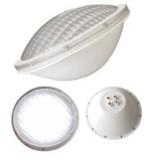
Power:21W Voltage:AC/DC12V Color:White,Red, Green, Blue, Yellow. LED Type: 48 pc SMD5730 LED Chip Size: Ф177mm x H106mm Material:Plastic + Transparent PC cover IP Rate:IP68 Beam Angle:120° Packing:20PCS/Carton
