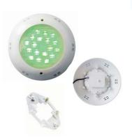
Power:25 W Voltage:AC/DC12V Color: White, Red, Green, Blue, Yellow. RGB LED Type:High Power Size: Ф290mm x H150.60mm Material: ABS + Transparent PC cover(lens)
