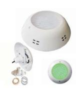
Power:18±1W(W/G/B)/17±1WRGB)/13±1W(Red) Voltage:AC/DC12V Color: White, Red, Green, Blue, Yellow. RGB LED Type:315PCS \* SMD3528/DIP F5 LED Chip Size: Ф290mm x H150.60mm Material: ABS + Transparent PC cover(lens) IP Rate:IP68 Beam Angle:120° Packing:10PCS/Carton
