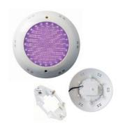
Power:18 $\pm$ 1W(W/G/B)/17 $\pm$ 1WRGB)/14 $\pm$ 1W(Red) Voltage:AC/DC12V Color: White, Red, Green, Blue, Yellow. RGB LED Type:105PCS 5050SMD Size: Ф290mm x H150.60mm Material: ABS + Transparent PC cover(lens) IP Rate:IP68 Beam Angle:120°
